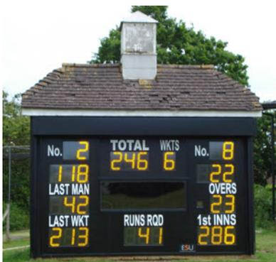
The new fascia was constructed in our factory and transported to the site. On day one our carpenters removed the old equipment and fascia and installed the new fascia and removable scorers window. On the second day P & I Protection fitted the electric roller shutter allowing us to install the electronic equipment on the third day.
